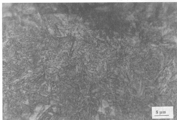
Fig. 5. Taper-section of a sandblasted specimen showing a lath martensitic microstructure in the surface layer.
